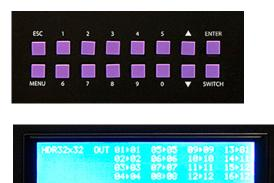
The MXCore-UD front panel enables one to switch directly from the Matrix without the use of any software.
