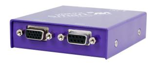
**Enhance VGA distribution and** extension via CAT5 cables at distances up to 1000 feet
