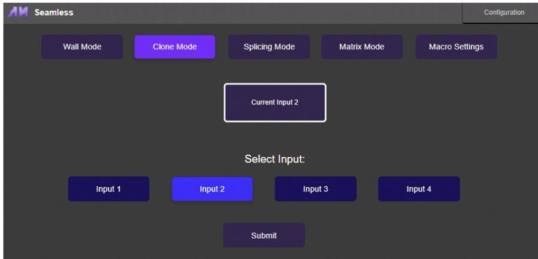
**Splicing Mode:** Select the desired input and preset and then click Submit. This will set QWALL-HD to “splice” the monitors to the selected input and preset. For example, if the user selects Input 1 and selects preset 1x2 (1+2), this will display Input 1 over Output 1 and 2. The user can then select Input 2 and select preset 1x2 (3+4) to display Input 2 over Output 3 and 4. There are many options available to use, and can even be used in conjunction with Matrix Mode.
