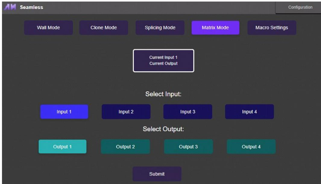
**Macro Settings:** This page allows the user to actively select and save presets onto the macro buttons found on the front panel. Button 7 is assigned by Macro 1 and button 8 is assigned by Macro 2. Simply select a desired preset, assign it to a macro button, and click Submit. This will allow the user to quickly use any “splicing” preset. Please note that the preset will also use the latest Input sent to QWALL-HD. Simply use button 1-4 to switch into any Input after using the macro button.
