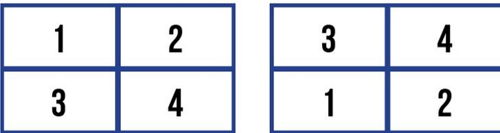
**Splicing Mode:** User can splice the input to do different matrix arrays (i.e. 1x2, 2x1, 1x3, 3x1, 1x4, 4x1).
